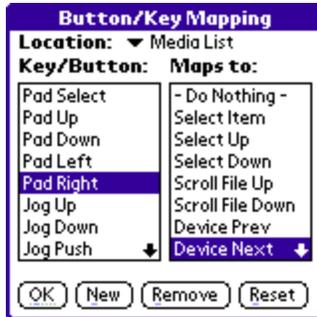
Accessible from a “Buttons” menu options, the TealPoint standard Button Manager provides a powerful and flexible interface for customizing the hardware button and key mappings for TealPoint applications. Mappings can be individualized for different locations (screens) in the application, and mappings can be created to support new buttons, jog-dials, and directional pads on future devices.
