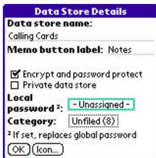
With 5-way controls, a current button, checkbox, or text field control is highlighted in blue-green or drawn bolded in monochrome handhelds. The current control is changed by presses of the directional pad, which moves the selection to a control in the general direction of the button press. The center “select” button will activate the highlighted control, pressing buttons, toggling checkboxes, or turn on or off the cursor in a text entry field.
