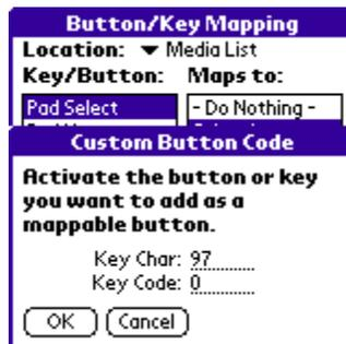
To create a mapping for a new key or button which is not listed, tap on the *New* button to bring up the custom code dialog. Press the button or control to be mapped, to capture the character its corresponding PalmOS key codes, and tap *OK* to create the key.
